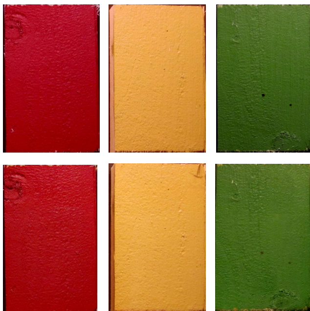
Fig. 3. Upper row: Samples imaged before the exposure (0 h). Lower row: Samples imaged after 1000 hours of the exposure. Samples from left: 29, 31, and 35.
