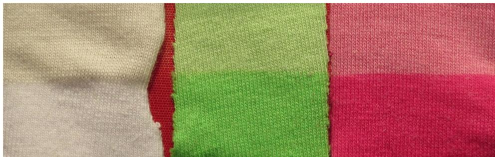
**Fig. 7.** Fading of the white, green and red Cotton fabric caused by the UV-A exposure. Upper part of the fabric was exposed.
