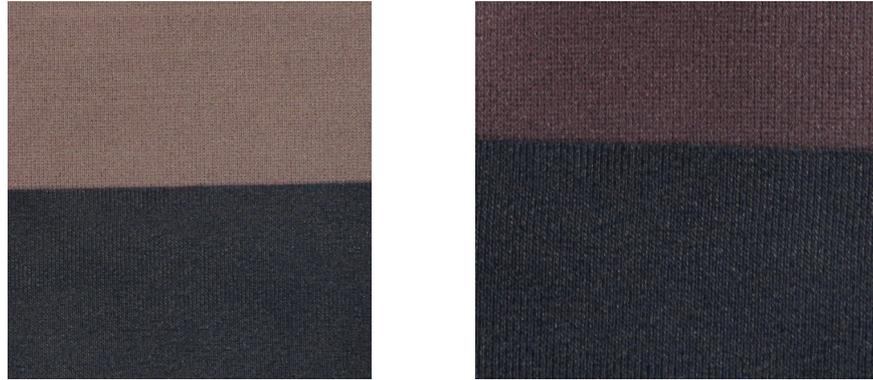
**Fig. 5.** Fading of the TommiDive blue shirt fabric caused by the UV-A (left) and solar (right) exposure. Upper part of the fabric was exposed.
