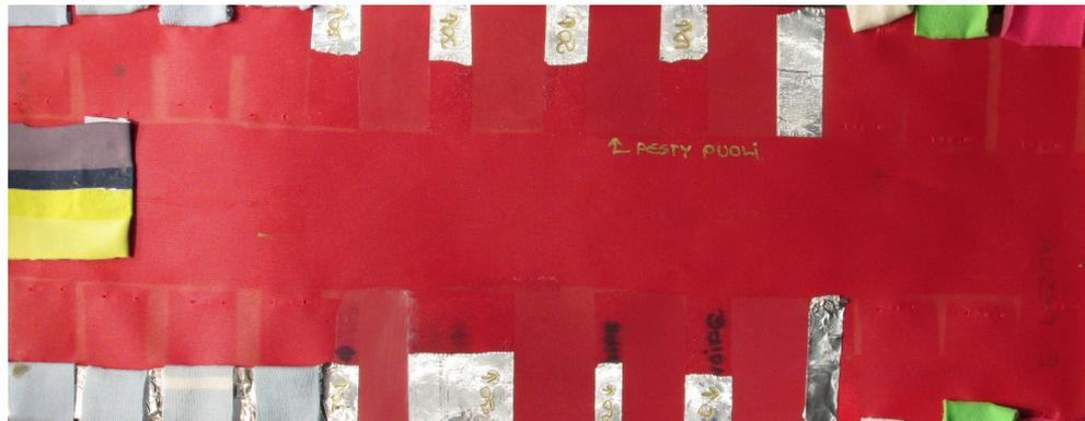
**Fig. 8.** Colour fading of the light sensitive red sail fabric under different protection (fabric or sunscreen). UV-A exposure.
