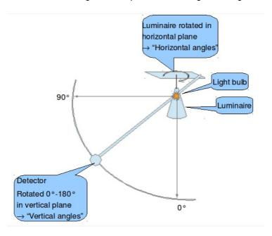
Fig. 2. Scheme of the test arrangement.
