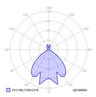
Fig. 4. Light distribution curve of Octo 4240. Since the luminaire is symmetric the light distribution curve is similar at every C-planes. Only the C-plane 0° is presented.
