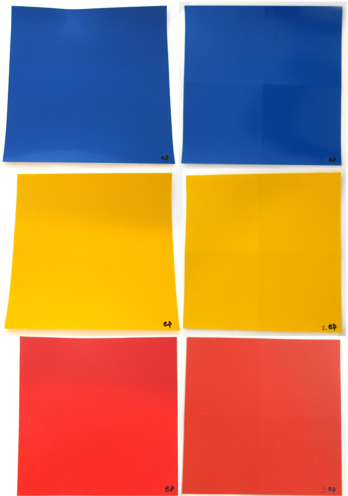
Fig. 4. Specimens before (left) and after (right) the low temperature crack procedure. From top: Vinyplan 6764, Vinyplan 6571 and Vinyplan 6581.
