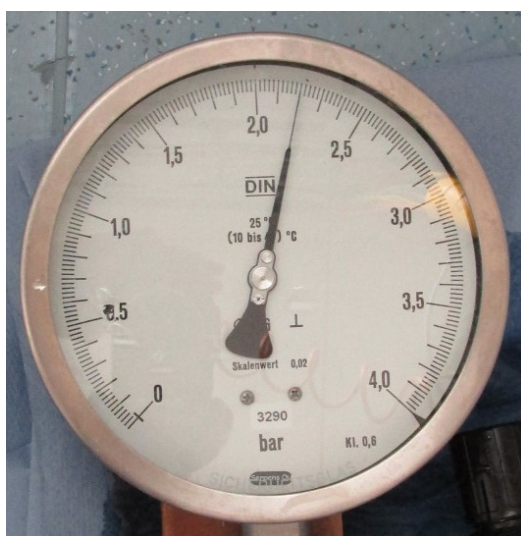
Fig. 6. Pressure gauge showing the maximum water pressure applied to the specimens.
