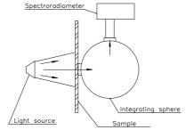
UVB range of the solar radiation is defined from 295 nm to 320 nm and UVA range is defined from 320 nm to 400 nm. The visual range is defined from 400 nm to 760 nm. In this test the visual transmittance measurements were done to the wavelength of 800 nm.
