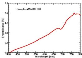
The UV transmittance of the fabric  $6776\ 099\ 820$  started at the wavelength of  $398\ nm$ . However, the UV transmittance of the fabric was still at  $400\ nm$  only  $0.0005\ \%$ . The mean visual
