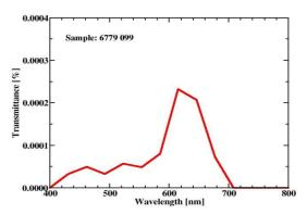
The UV transmittance of the fabric 6779 099 was 0%. Also at the visual wavelengths the mean transmittance of the fabric 6779 099 was only 0.0001% which can be approximated to be 0%.
