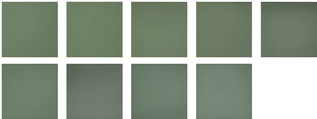
Nordic Green samples: Upper row from left, 0 h, 92 h, 168 h, 336 h and 426 h, lower row from left, 510 h, 702 h, 846 h and 1000 h.
