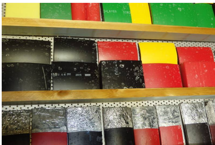
Fig. 2. Test arrangement showing the samples under solar irradiation during Exposure 1. Note: A larger set of samples was involved in the first part of the test (Exposure 1).
