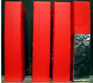
Fig. 7. Meritaito D800 samples after the exposure to UV radiation. From left: No. U5 (reference sample stored in dark at room temperature), No. U1, U2 and U3 (sample with foil strips).
