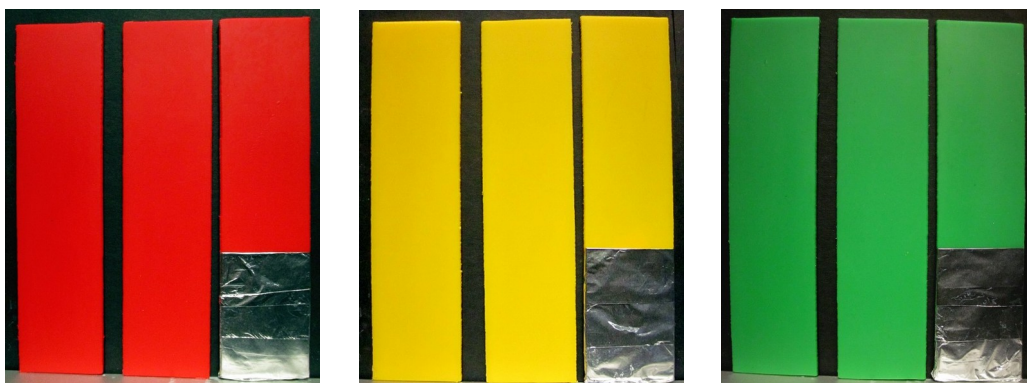
Fig. 9. RotationsPlast Red, Yellow and Green samples after the exposure to UV radiation. For each colour, from left: No. 3 (reference sample stored in dark at room temperature), No. 1 and No. 2 (sample with foil strips).
