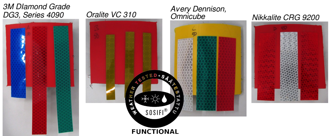
Fig. 1. One set of test samples, four different retroreflective sheetings, three pieces of each, prepared for the test.
