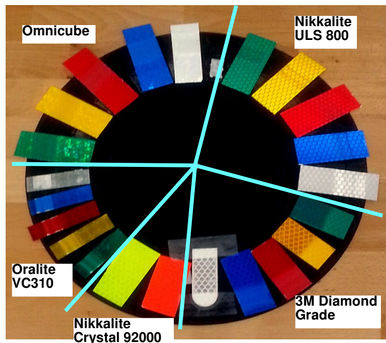
Fig. 2. Test samples. Omnicube, Nikkalite ULS 800, 3M Diamond Grade and Oralite VC310 reflector materials in colours green, yellow, red, blue and white, and Nikkalite Crystal 92000 reflector material in colours fluorescent yellow and fluorescent orange were tested.
