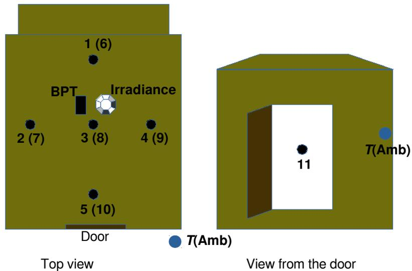
**Fig. 6.** Placement of the temperature and irradiance sensors shown schematically.
