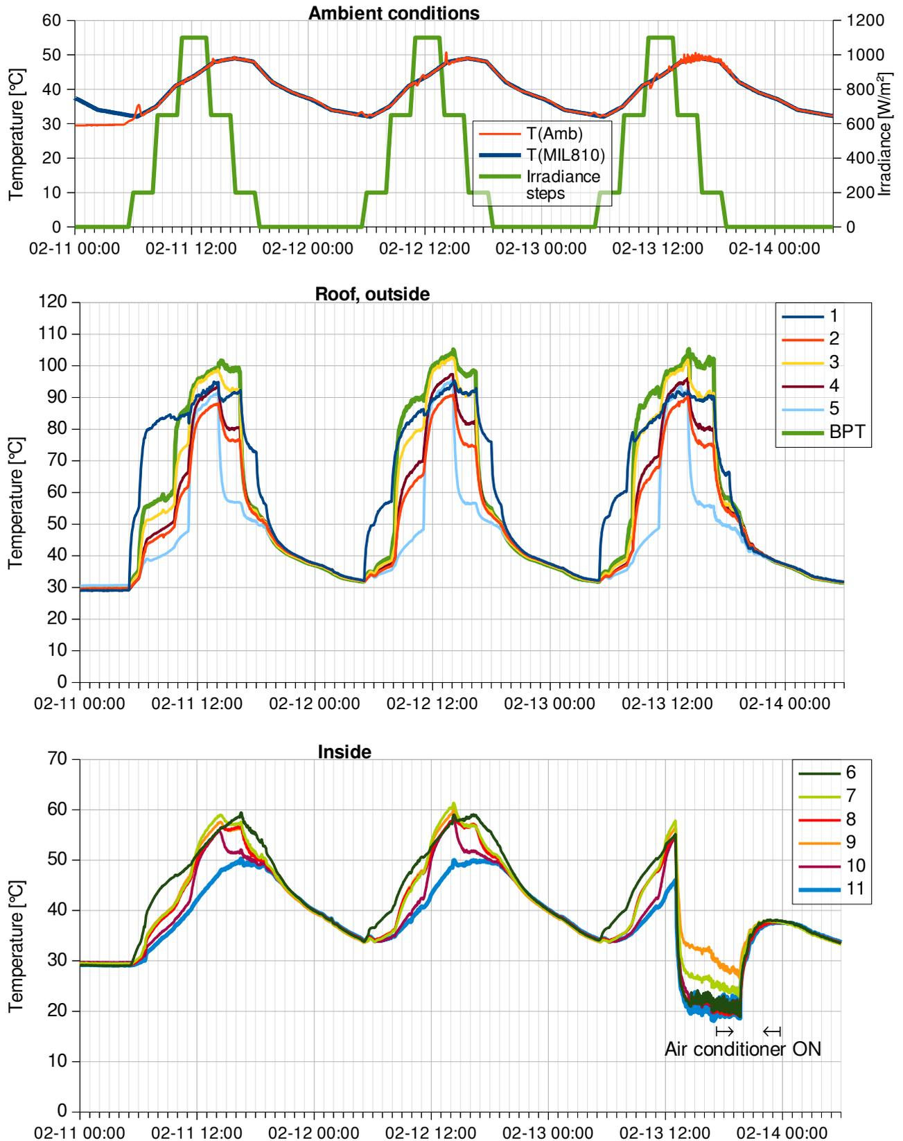
**Fig. 9.** Temperatures measured at positions No. 1 – 11 (as indicated in Figs. 6 and 7), and the ambient temperature and irradiance conditions.
