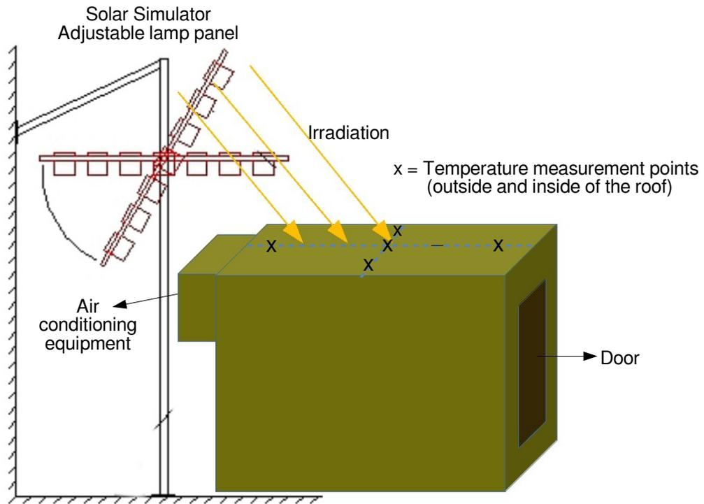
**Fig. 4.** Schematic representation of the solar testing arrangement.
