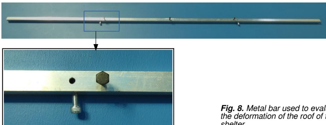
**Fig. 8.** Metal bar used to evaluate the deformation of the roof of the shelter.
