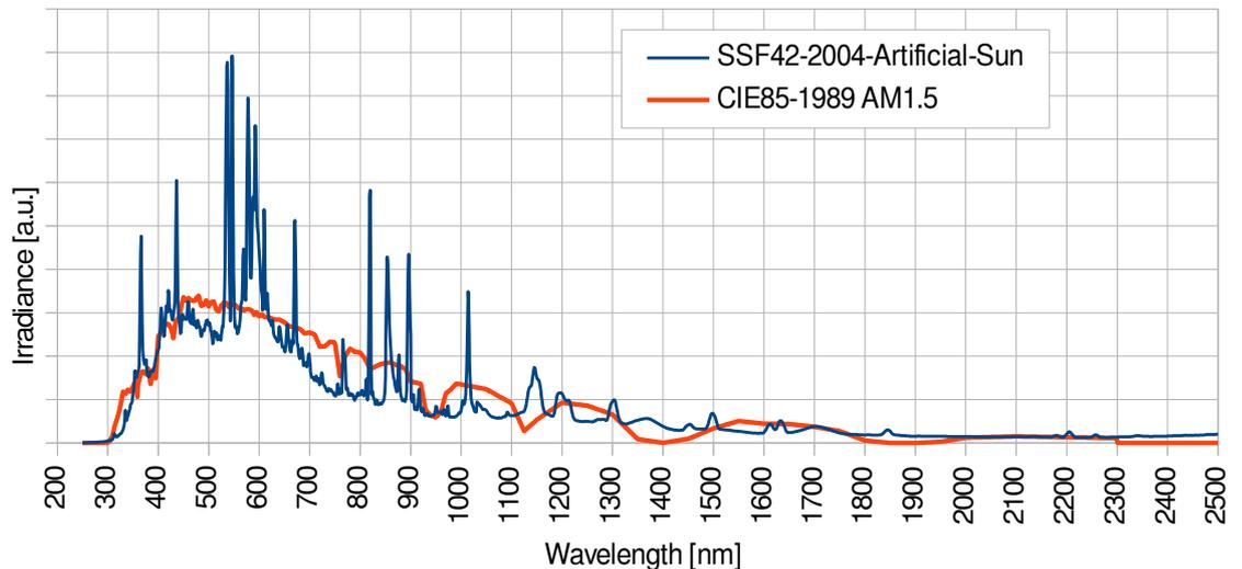
**Fig. 3.** Spectrum of the simulated solar radiation used in this test (blue curve) and spectrum of natural sunlight according to CIE 85-1989 (red curve). The spectra are scaled to the same total intensity.
