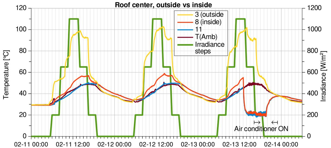
**Fig. 10.** Surface temperatures measured at the center of the roof; outside (sensor No. 3) vs inside (sensor No. 8). It can be seen that the difference between the outside and inside surface temperatures was 40°C – 45°C when the ambient temperature and irradiance were high. When the air conditioner was operating, the corresponding surface temperature difference was 70°C – 80°C. Sensor No. 11 shows the ambient air temperature inside the shelter.
