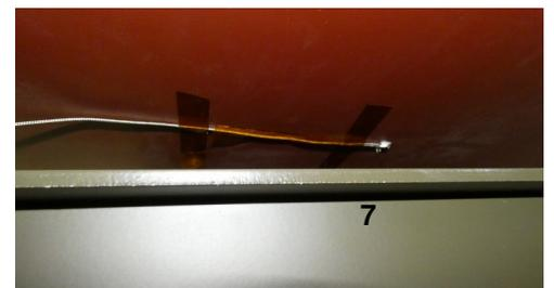
**Fig. 7.** Placement of the temperature and irradiance sensors. Heat-conductive adhesive was used to attach the sensors to the shelter surface, as can be seen in the close-up image of sensor No. 10.
