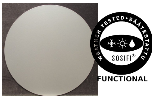
Fig. 1. Sample under test, Normastic 405, Grey, painted on a circular plate.
